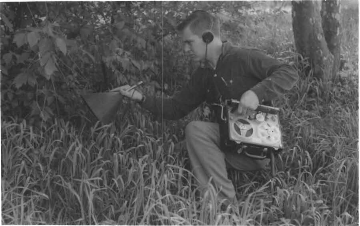
Fig. 26. Recording a ground cricket ( Nemobius sp.) at close range in the field with microphone inside funnel.
